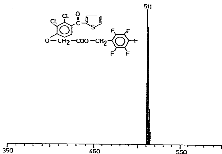
Fig. 3. Mass spectrum of tienilic acid after derivatisation with pentafluorobenzyl bromide and gas chromatography (chemical-ionisation mode).
